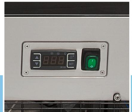
Digital temperature controller on backside
