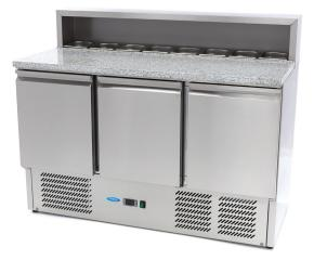
Robust worktable with 3 stainless steel doors Stainless steel top with granite work area Inside and outside in stainless steel AISI 304 Capacity 400L Capacity for 8 x 1/6 GN Including adjustable shelves (one per door) Dixell digital temperature controller Cooling system with fan Foamed evaporator on 3 sides Automatic defrost Zanussi compressor Refrigerant R290 / CFC-free Insulation thickness 35 mm Temperature: 0 ° to + 10 ° degrees Celcius
